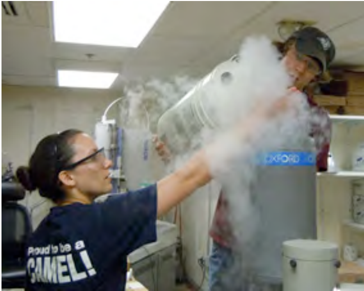
In the Ching group, Kathryn Tutunjian '13 and Ian Richter '14 pour liquid nitrogen into the SEM EDAX detector while Jeff Carchmichael '14 operates the SEM.
